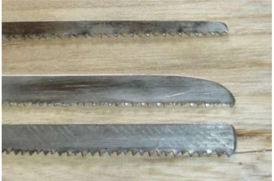
Band-saw blade stock is a good starting point for making frame saw blades and pad saw blades. If you have a band saw, you may have a collection of broken and blunt blades that you may be wondering what to do with. If not, they are probably available for the asking. The used blade shown below is a 19mm wide, 3 tpi blade that broke at the weld after some use. The stock is 1mm thick.
