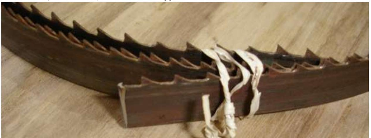
3. The blade needs to be cut to length and holes drilled.
