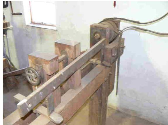
that gouges rather than hook tools were used although no turning chisels remained. The next picture illustrates the tool-rest and the headstock. The swing is about 380 mm and the bed length 1.8 metres. Unfortunately we could not find a drive spur for the headstock. It was suggested that the owner obtained tools that were used by patternmakers in the Reef foundries. It is interesting to note that the tool-rest is set on
