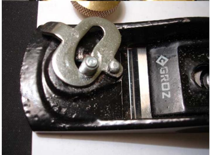
back to close up the mouth, but it leaves an unsightly gap in the front, with some sharp points exposed. The Groz is on the right, and the Stanley on the left. Groz changed the design slightly, but clearly, somebody did not get their sums right. I removed the sharp edges by grinding the front of the sole as shown in next the picture on the left. (I wonder whether the sole plate was not inserted the wrong way around, before being ground to fit?)
