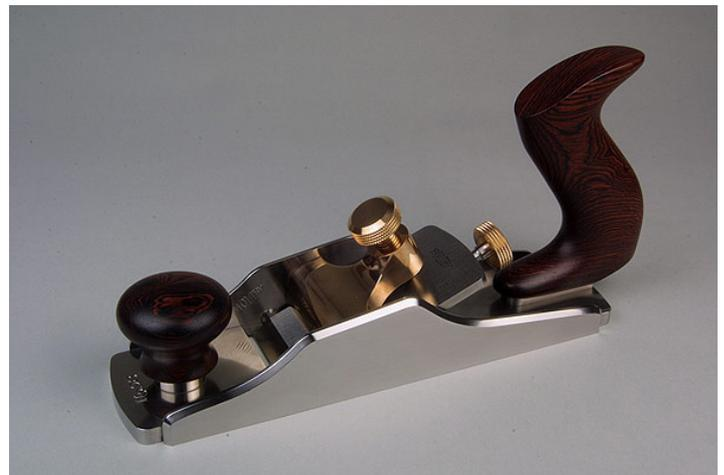
Holtey says the thicker steel used for the body more than compensates for the loss of rigidity lost from the lack of an infill.
