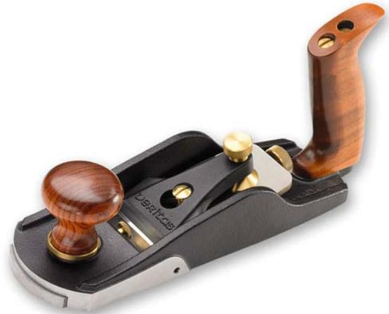
The 982 (shown bottom, right) has a more conventional blade location, with the bevel down. The bed angle is  $55^{\circ}$ , commonly called the York pitch, also suited for difficult grain. The adjuster follows the same principle as the Norris one, but has been improved to be smoother under higher clamping loads. The body is also made of thicker steel, to be 40% heavier.
