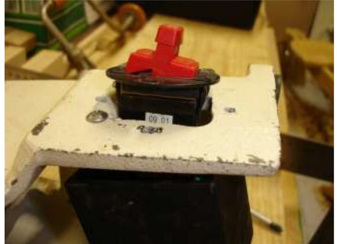
A **No-Volt-Release** motor starter is an electromagnetic relay for starting and stopping a machine. When selecting a motor starter, it is important that the starter is correctly rated for motor power. This is because induction motors directly connected to the supply at start-up draw a much higher current than listed on the nameplate until they get up to speed, and the starter contacts need to be rated to supply this.
