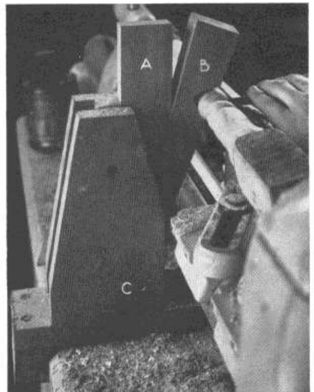
FIG. 8. SIMPLE WOOD STEADY MADE FOR MYFORD LATHE. The idea could be adapted to suit any make of lathe. (A) is the wedge which tends to drop down by gravity and keep the slip (B) up to the work. The slip is pivoted at C).
