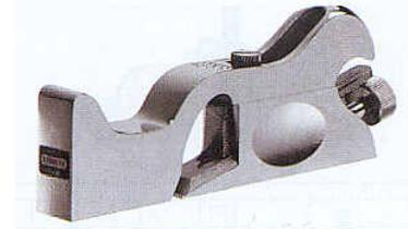
The No 78 can be used for making fine adjustments to tenons, but if you have one, a shoulder plane (Stanley No 90, No 92 (see right) or No 93 or equivalent) with a finely set mouth and low blade angle may be better. To fine tune the width of a groove a Stanley No 79 side rebate plane can be used after the No 78 has done the heavy cutting.
