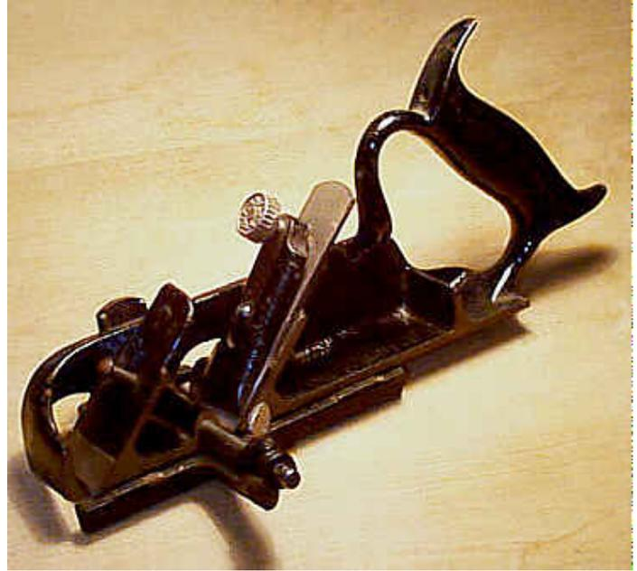
There is an adjustable depth stop on the right hand side of the plane, secured in place by a thumb screw. Directly below the depth stop, is a three-pronged spur to score the grain that sits flush with the side of the plane. It can be turned up out of the way when it isn't needed. There is no spur on the left of the plane.
