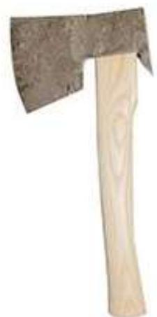
The traditional side axe has a wide blade with the bevel on only one side and a short handle. The handle may even be offset slightly to provide clearance for working close to a flat surface. I have not seen any of these specialised axes for sale locally.
