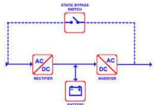
The 7 Ampere – hour (Ah) rating of the batteries refers to the capability of the batteries to supply a certain amount of energy. The Ah rating is usually calculated at the 20 hour rate – the current drained to discharge a fully charged battery over a period of 20 hours. In this case,  $7Ah \div 20 = 0.35 A$  for 20 hours. Discharging the battery at 0.35 amps for 20 hours gives you 7 Ah. The output voltage is approximately 12 V, so  $12V \times 7Ah = 84$  Watt hours (Wh) of energy.
