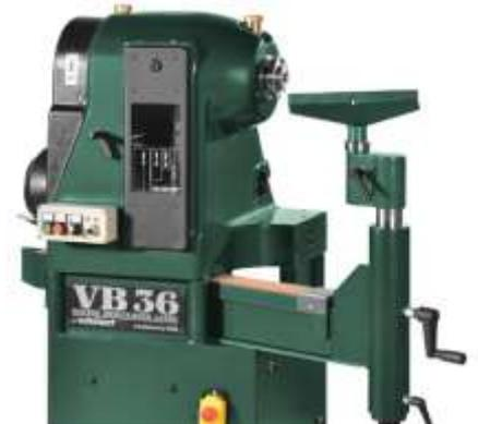
All the lathes mentioned below accept 2 Morse Taper (MT) tooling and most have a 1" x 8tpi headstock spindle thread. Accessories in these sizes are widely available. The larger Novas and Jets may have larger spindle threads, so check this before you upgrade.
