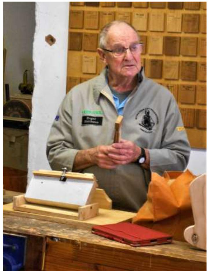
Eugene showed a set of jigs for holding sash cramps when gluing up jointed boards. It not only holds the cramps but there is also provision for space to use G-Clamps for holding down the work. A very useful set of jigs, which are simple to make.
