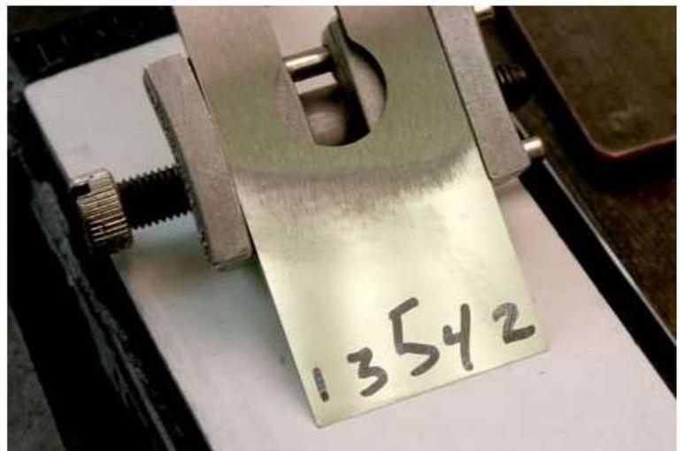
I start with the #1,000-grit waterstone. This stone cuts quickly enough to shape an edge or remove small nicks or chips. Clamp your cutter in your honing guide then (mentally) divide its edge into five “positions” (see the photo above for details).
