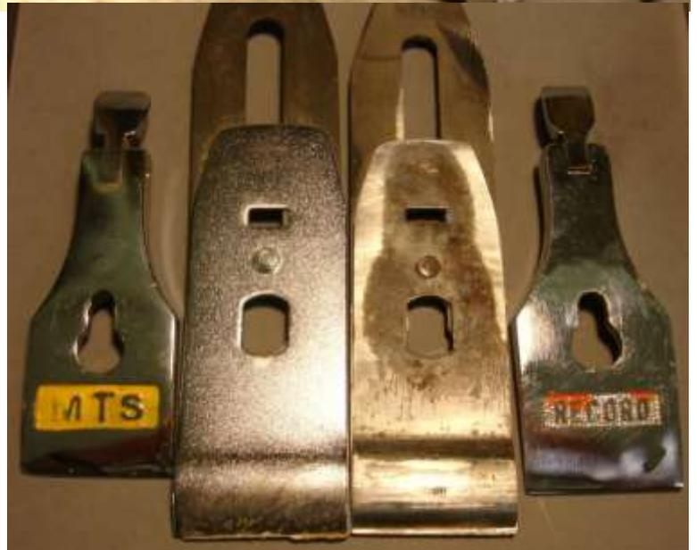
The combination of these latter three flaws means that when the plane is used, vibrations from the cutting forces can cause the lever cap to move backwards and pop off, as Steven has experienced.
