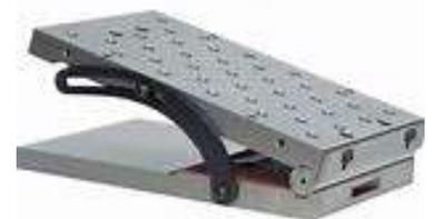
The principle of a sine plate is illustrated in the diagram below. The equation given allows you calculate the height of the spacer Z required between the two boards on the left-hand side. For those who require a quick refresher for high-school trigonometry, you may remember the equation
