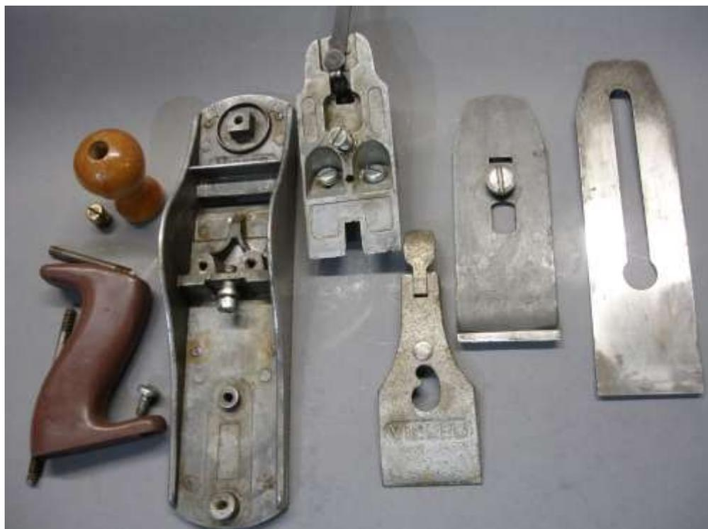
I removed the handles and supported the plane upside down on two blocks of wood at each end, where the handles were attached. Using a hard rubber mallet, I then carefully hammered around the mouth area, to try to bend the sole very slightly. Using increasingly hard blows, and measuring the straightness after each one, I was able to reduce the
