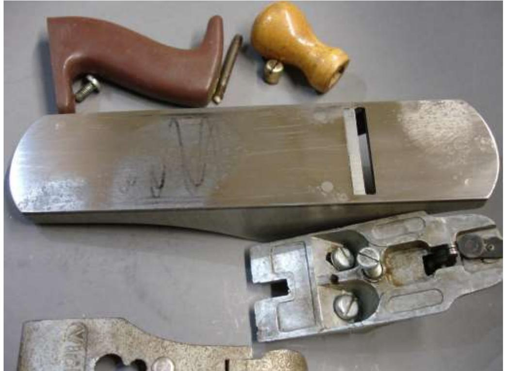
Once the sole was reasonably flat, I fettled the cap iron front edge and sharpened the blade. The back of the blade was not too curved - it took about ten minutes of work on the diamond plate get it to an acceptable flatness. There was quite a significant wire edge when sharpening, so I suspect the blade is not quite as hard the Stanley blades I am used to.
