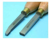
available are 20 threads per inch (tpi), 18 tpi, 16 tpi, 12 tpi and 10 tpi (See http://www.toolpost.co.uk/pages/Turning Tools/Thread Cutting/thread cutting.html). Fine grained woods such as box or fruit woods give the best results. Jacaranda will also do, with care. Buddy showed some special tools he has made to make the work easier, including a recessing tool to relieve the inside end of the thread.
