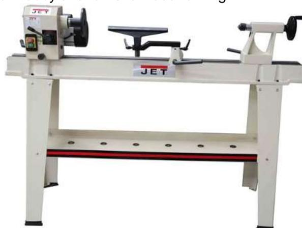
Centre. A Reeves drive uses a belt between two cone pulleys – by moving the speed control lever, the relative diameters of the two pulleys are changed, giving a range of speeds. The speeds can only be changed while the lathe is running, which can be a disadvantage. If you have mounted a large workpiece and realise that the speed is set too high, then for safety, you may have to remove it before running the lathe and moving the speed control lever to minimum, before remounting the piece.
