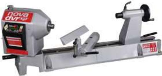
Some people would prefer solid switches and an analogue speed control knob. Fitting a surge plug is apparently a wise precaution, given our high lightning incidence in Gauteng, and the poor power quality experienced by some consumers. This applies to all lathes with electronics, not just the DVR.
