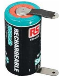
I selected and bought 12 Sub C cells from RS Electronics at R38- ea plus VAT = R520-. Not cheap, but the new replacement drill from AEG that is roughly equivalent to mine is about R1500-, so I thought it was worth doing. These cells are NiMH with a capacity of 3000mAh as shown on the right. They come with tags that can be soldered.
