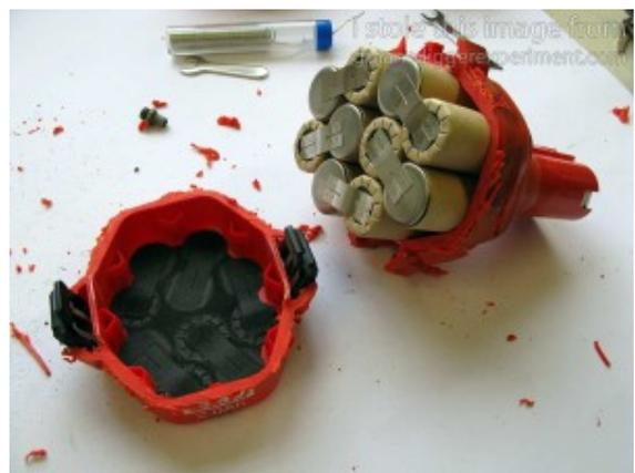
Count the number of cells, and measure the size. A typical size is Sub C which is about 22.5mm diam by 43mm high. This is important to ensure that the batteries will fit into the case once they have been assembled into a pack. There are several sizes, so you must check.
