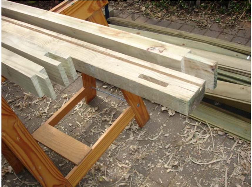
For the top rail, I joined the posts to the rail, using blind mortises in the underside of the rail and tenons cut on the top of the posts. The posts were joined to the lower rail using a bridle joint. The upper surfaces of both rails were chamfered, so as to shed water. The cladding was housed into a slot on the underside to the top rail for mechanical support. The length of cladding used made it quite flexible, so housing one side in the groove provided support.
