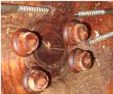
Fortunately, the screw holes were covered with neatly made plugs which were easy to prise out. The glue used appears to be Cascamite, which is a water-proof glue with some gap filling properties. It is also quite brittle, so a sharp knock was all it took to dislodge the plugs. With the plugs removed, and the screws withdrawn, the loose two legs were removed. A light tap with a mallet was all it took to dislodge the fourth.
