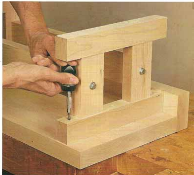
Attach the base. Mount the top to the base by driving three screws through holes (two slotted, one round) in each apron.
