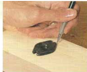
Inset the veneer-press nuts into the back of the bench face. Trace the flange profile (above) and rout a recess to set the nut flush with the stock. Secure with screws (below).
