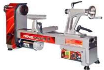
The belt cover swings up to expose the belts, so changes can be done by sight and not feel. Low speed torque is adequate on the lowest belt speed, except with the largest workpieces, when a very light cut will be required. It has a spindle lock/indexer and weighs about 40 kg. It has the usual 1" x 8 tpi head stock spindle thread and #2 MT sockets in the headstock and tail stock.
