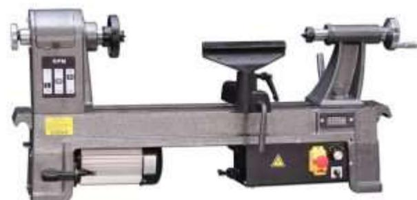
motor, with a variable speed inverter, which combined with three pulley ratios has a speed range of 100 to 4000 rpm. Due to the inverter drive and larger motor, the slow-speed torque is likely to be much more substantial than the DC motors of the smaller models. The spindle thread is the widely used 1" x 8 tpi with #2 MT sockets in the head and tail stocks. The increased capabilities are reflected in the price of R15200-.
