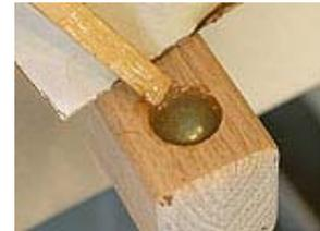
Insert the bolts through the bottom caul halves; add a couple flat washers and a nut.
