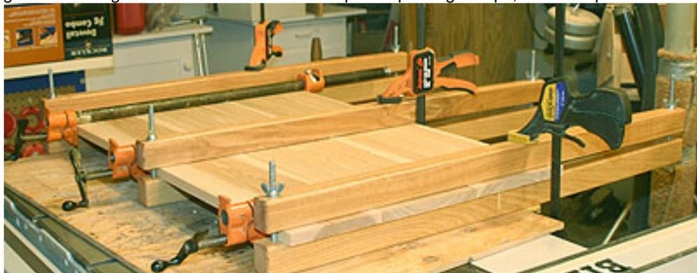
The important features of clamping cauls are rigidity, length and width. The overall length of a caul impacts its ability to resist flexing
