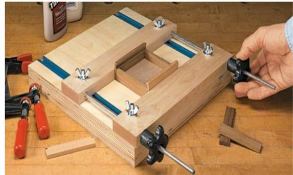
To use the clamp, loosen the wing nuts and place the parts to be clamped between the blocks. Position the front of the clamping block to extend slightly beyond the edge of the base so you can turn the knobs and secure the stop block in place. Finally, snug up the star knobs and tighten the wing nuts to lock the clamping block in place.
