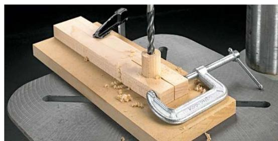
Build the jig by first drilling a hole the diameter of the dowel in a piece of hardwood. Then just cut a saw kerf through the hole from the end to make a clamp.
