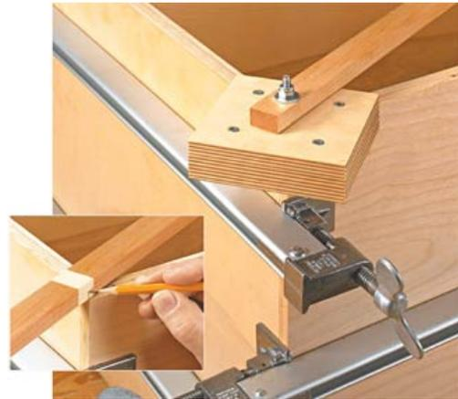
The jig makes it easy to work from the far end of a frame or case. You first slide the block over the corner and it hooks into position. Then just extend the long measuring arm diagonally across to the opposite corner.
