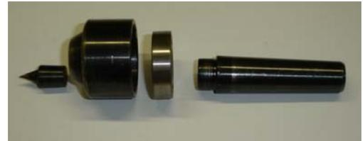
The example of false economy that I have in mind is the bearing fitted to the live centre supplied with my Jet 1014 Mini lathe (2004 vintage). The Jet live centre is a cheap and simple design that is also versatile.
