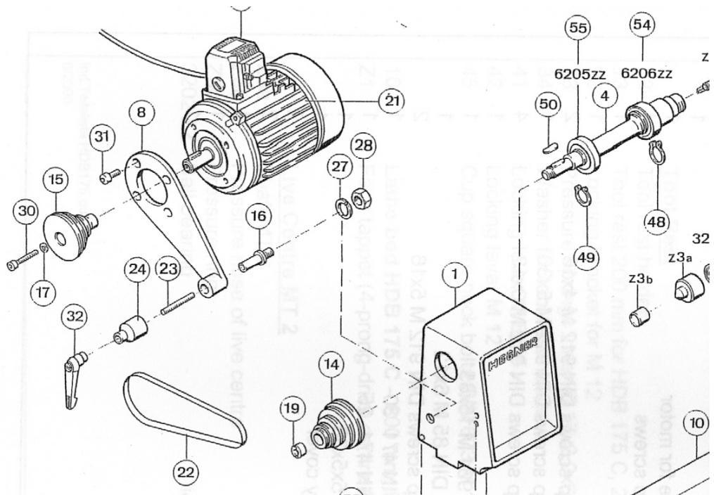
shim to take this up. The shim was fitted on the side of the keyway (50) for the pulley.
