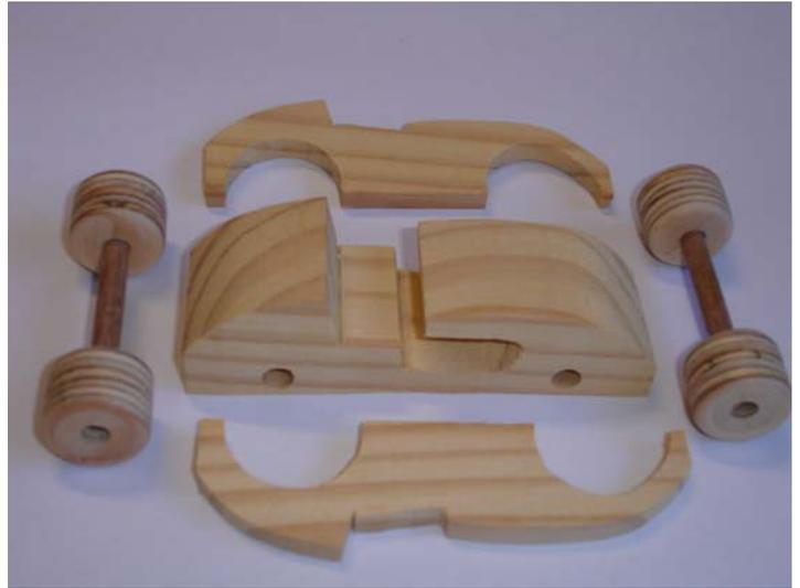
2. Sketch out the overall shape on a rectangular block of wood – the starting piece of wood for this model was 110 mm long x 48mm wide x 36 mm high of SA Pine. (A piece of  $4\frac{1}{2} \times 1\frac{1}{2}$ " = 114 x 38mm S5 grade pine can be used to make a lot of cars.) The limitation in this case was that the width had to fit the maximum size that the scroll saw can handle.
