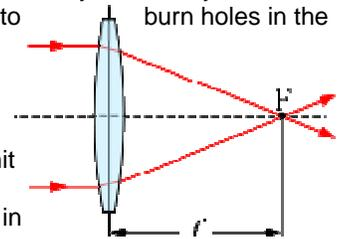
One benefit of quantifying a lens in terms of its optical power rather than its focal length is that when [relatively thin lenses](#) are placed close together their powers approximately add. Thus a thin 2-dioptre lens placed close to a thin 0.5-dioptre lens yields almost the same focal length as a 2.5-dioptre lens would have.
