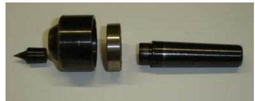
The hollow shaft is a useful feature, because it allows drills to be inserted through the tailstock to bore a hole in the work piece. When making tool handles for tools that have a tang that locate in a socket in the handle, the hole can be bored concentrically, without removing the work piece from the lathe. Clearly some thought went into the design of the Jet live centre. However, I think some cost cutting production engineer then spoiled things by installing the wrong bearing in my one.
