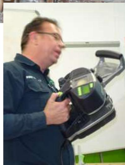
edging up to 2mm thick. The edges can be straight or curved – inside or outside, down to a radius of 50mm. The unit is fully automatic, self-feeding with a short warm-up time. You will need to budget R56k for a unit that includes accessories in a Systainer, so only larger shops will be able to justify it. The top picture shows the size of the unit. The lower picture shows Martin attaching a 2mm edging to a curved chipboard edge.
