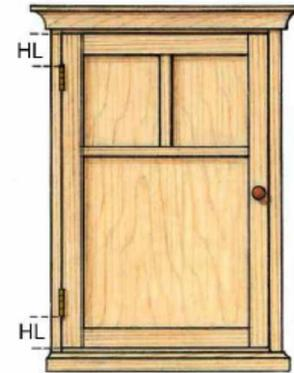
If rails narrower than length of hinge then use length of hinge (HL)
