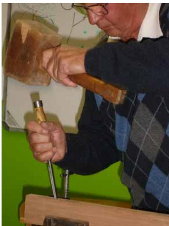
traditional technique for making a mortise and tenon joint: chopping the mortise by hand using a mortise chisel and cutting the tenon using a tenon saw.
