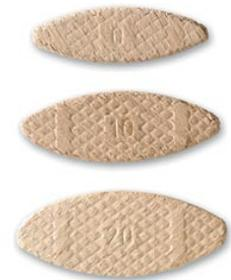
Biscuits were designed for joining man-made boards, such as chipboard. They are made from compressed beech, with the grain running at a diagonal to the long axis. They provide a good surface area to make strong glued joints, so they work well in weaker materials. Chipboard is weak compared to natural wood, even compared to softwoods such as SA Pine, so the larger glue area compared to round dowels works
