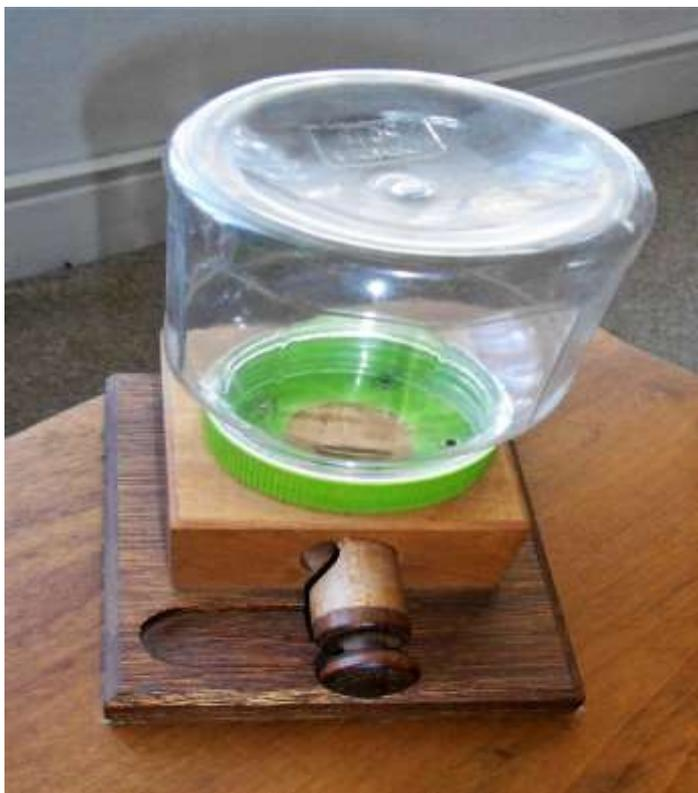
◀ Glenn showed us his "Gum Ball" dispensing machine, better known in the USA than here. He explained how the jar is filled with chewing gum balls, and the balls are transferred from the jar to the receptacle by pulling the protruding knob, which has a spiral inside which runs on a pin and turns as it is pulled out depositing the ball in the groove on the base.
